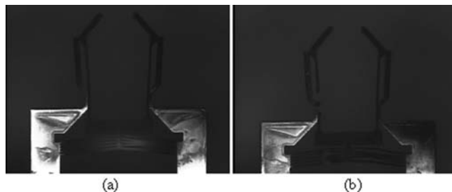
Fig. 10a,b. Optical photomicrographs of the design 2 metallic microgrippers with excessive voltages applied ( > 4.5 V). a A burning microgripper; b a completely burnt and structurally disintegrated metallic microgrippers
