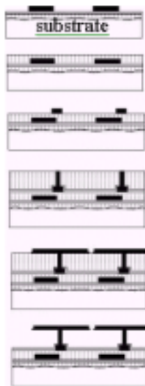
Fig. 3. Fabrication procedures for micromachined mirror arrays on low cost substrates.
